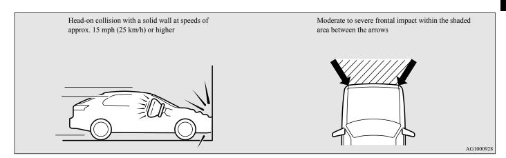
The front airbags and driver's knee airbag are designed to deploy when the vehicle suffers a moderate to severe frontal impact. A typical condition is shown in the illustration to the left.
