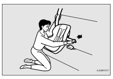
3. To activate the ALR child restraint installation function, slowly pull the shoulder part of the belt all the way out of the retractor until it stops. Then let the belt feed back into the retractor.
