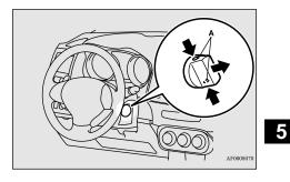
3. Insert the emergency key into the ignition switch, and slowly push and turn.
