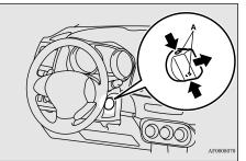
4. Insert the emergency key into the ignition switch.
