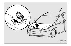
Support the engine hood with the hood prop. Insert the hood prop securely in the opening under the hood marked with an arrow.
