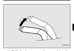
1- Pull the lever up without pushing the button at the end of hand grip.
