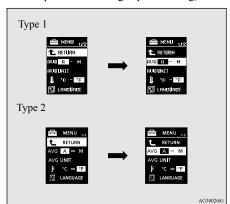
3. Press and hold the multi-information meter switch (for about 2 seconds or more) to switch in sequence from A or 1 (Auto reset mode)  $\rightarrow$  M, 2 or P (Manual reset mode)  $\rightarrow$  A or 1 (Auto reset mode). The setting will change to the selected mode condition.
