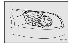
2. Pull the cover out in the direction of the arrow shown in the illustration.
