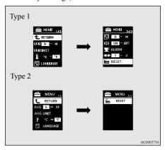
3. Press and hold the multi-information meter switch (for about 5 seconds or more), the buzzer sounds and all of the function settings are returned to the factory settings.
