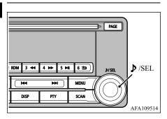
1. Select "YES" at the "Adjust time" screen, and press the ▶/SEL key.
