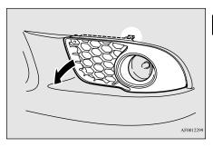
3. Remove the screws (B) and pull the entire light unit out.
