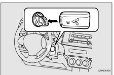
5. Turn the emergency key with the F.A.S.T.-key to the "ON" position for 5 seconds.
