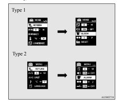
3. Press and hold the multi-information meter switch (for about 2 seconds or more) to display "ALARM" (rest time setting).
