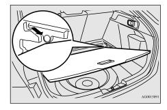
3. Push the board in all the way with the front part lowered, then set the board into place.
