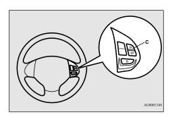
To increase your speed in small amounts, press the "ACC RES" switch for less than about 1 second and release it.
