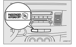
The indicator normally comes on when the ignition switch is turned to the "ON" position and goes out a few seconds later.
