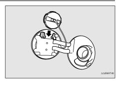
5. To fill with fuel correctly depends mainly on correct handling of the fuel filler nozzle. Do not tilt the nozzle. Insert the nozzle in the tank port as far as it will go.
