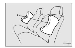
A label is attached to the seatbacks in vehicles with side airbags.
