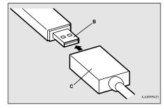
4. Connect the USB connector cable (C) to the USB input terminal (D).
