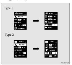
3. Press and hold the multi-information meter switch for about 2 seconds or more to switch in sequence from 1 (turn signal sound 1)  $\rightarrow$  2 (turn signal sound 2)  $\rightarrow$  1 (turn signal sound 1).
