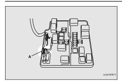
3. Clamp it on the fuse you wish to remove, and pull the fuse straight out from the fuse block.
