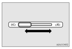
If the outside air is dusty or contaminated in some way, use the recirculation position. Switch to the outside air position every now and then to keep the windows from fogging up.
