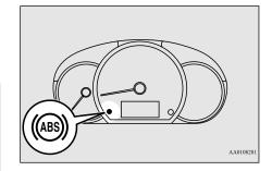
If there is a malfunction in the system, the anti-lock braking system warning light will come on.
