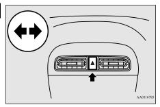
If you press the flasher switch, the turn signals will flash intermittently, and so will the hazard warning lights. This is an emergency warning system and should not be used when the vehicle is in motion, except for emergen-
