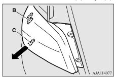
4. Turn the socket counterclockwise to remove it.
