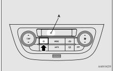
Push the switch again and the air conditioning compressor will stop and the indicator goes off.
