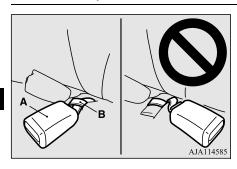
2. Route the seat belt through the child restraint system according to the instructions provided by the child restraint system's manufacturer. Then insert the seat belt latch plate into the buckle. Make sure you hear a "click" when you insert the latch plate into the buckle.
