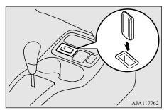
4. With the first valid F.A.S.T.-key, press the UNLOCK button for 4 to 10 seconds and press the LOCK button during this time.
