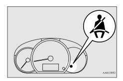
If the ignition switch is turned to the "ON" position or the operation mode is put in ON without the driver's seat belt being fastened, a warning light will come on and a tone will sound for approximately 6 seconds to remind you to fasten your seat belt.
