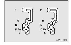
Set the selector lever in the gate to operate while the brake pedal is depressed.
