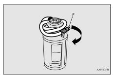
9. Pull out the compressor's hose (G) from the bottom of the compressor and securely attach it to the valve (H) of the bottle by turning it clockwise until tight.
