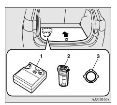
Tire repair kit which consists of 1 to 3.
