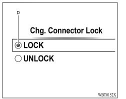
Turn the scroll dial (C) to select "LOCK" (D) and press the scroll dial (C) to confirm.
