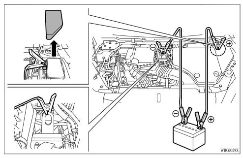
If the auxiliary battery runs out and you cannot turn on the power switch, ask for a rescue vehicle, connect the booster cable (sold separately), and start the Plug-in Hybrid EV system.
