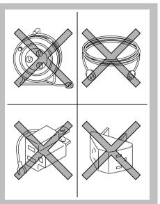
• To prevent an electrical shock or fire, do not use a multi type outlet. The grounded line may not work properly and it is not a dedicated type outlet.
