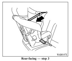
3. Pull the shoulder belt until the belt is fully extended. At this time, the seat belt retractor is in the Automatic Locking Retractor [ALR] mode (child restraint mode). It reverts to the Emergency Locking Retractor [ELR] mode when the seat belt is fully retracted.
