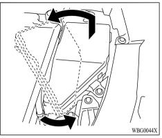
③ Slightly lift up the entire cover and rotate it slowly counterclockwise toward the EV unit cover while lifting up the rear part further, centering on the front edge of the cover.
