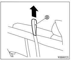
3. Pull the strap (B) and fold the seatback forward.
