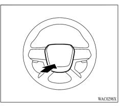
To sound the horn, push the center pad area  $(\mathbf{b})$  of the steering wheel.
