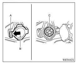
2. Press the tab (A) to open the inner lid (B).
