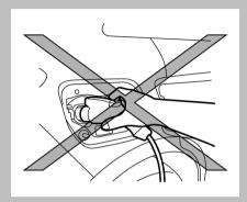
Do not grasp the top of normal charge connector. It could cause injury from the protrusion on the charging lid.
