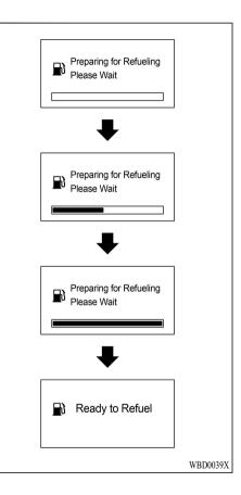
3. The internal pressure of the fuel tank will automatically be released to prevent fuel overflowing from the fuel filler.
