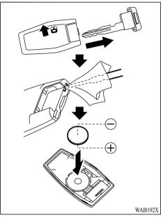
Replace the battery in the F.A.S.T.-key as follows:
