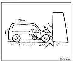
The driver and front passenger airbag and knee airbag systems will deploy in the event of an impact which exceeds a 16 MPH (25 km/h) frontal collision with a solid wall that does not move or deform.
