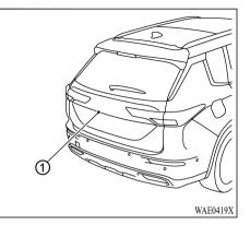
To display the rear view, the Rearview camera system uses a camera located just above the vehicle's license plate ①.
