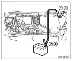
9. Connect the other end ② of the cable connected in step 9 to the positive terminal of the rescue vehicle battery.
