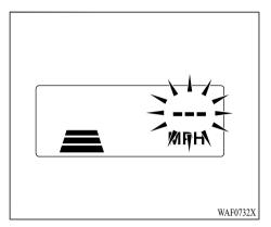
When the SET- switch is pushed down under the following conditions, the ACC Assist system cannot be set and the set vehicle speed indicator blinks for approximately 2 seconds.
