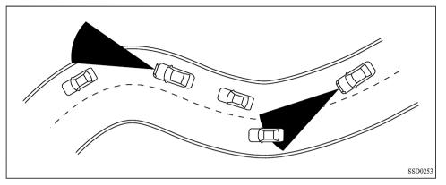
When driving on some roads, such as winding, hilly, curved, narrow roads, or roads which are under construction, the radar sensor may detect vehicles in a different lane, or may temporarily not detect a vehicle traveling ahead. This may cause the PFCW system to work inappropriately.
