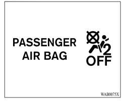
7. If the booster seat is installed in the front passenger seat, place the power switch in the ON position. The front passenger airbag status light \$\$\$ may or may not illuminate depending on the size of the child and the type of booster seat used. See "Front passenger airbag status light" (P.3-57).
