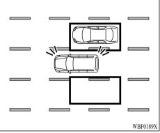
**Illustration 5 – Overtaking another vehicle** Illustration 5: The side indicator light illuminates if you overtake a vehicle and that vehicle stays in the detection zone for approximately 2 seconds.
