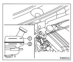
Check the fluid level in the reservoir. If the fluid is below the MIN line ② or the brake warning light comes on, add MITSUBISHI MOTORS GENUINE BRAKE FLUID SUPER4 (DOT 4) or conforming to brake fluid **DOT 3** or **DOT 4** up to the MAX line ①. If fluid must be added frequently, the system should be checked. It is recommended you visit a certified Mitsubishi EV dealer for this service.
