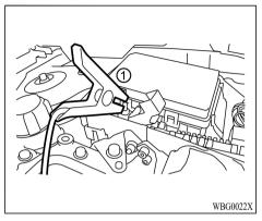
Open the rescue terminal cover in the fuse box of your vehicle while pressing the tab.
