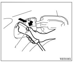
7. When the charging indicator (G) stops blinking, charging is complete. Pull out the normal charge connector while pressing the release button (J).
