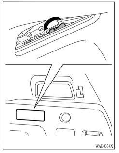
2. The normal charge connector is unlocked by turning the white dial, which can be seen from the underside of the cut out of the lid, counterclockwise about 12 times.
