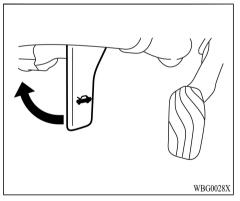
5. Pull the hood lock release handle at the bottom right of the driver's seat of your vehicle to open the hood.
