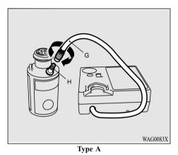
10. Install the bottle onto the compressor.
