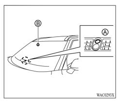
Be sure not to put anything on top of the light sensor (a) (if so equipped) located on the top of the instrument panel or rain/light sensor (b) (if so equipped) located above the inside mirror. The sensor controls the Auto Headlight; if it is covered, the sensor reacts as if it is dark and the headlights will illuminate.
