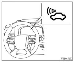
The Acoustic Vehicle Alerting System [AVAS] is device that uses sound to alert pedestrians of the presence of the vehicle. The system operates in the following cases when the engine is not running and the READY indicator is illuminated:
