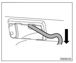
3. Then tilt the jack bar down to release the lock of the fuel filler door.
