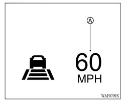
When passing another vehicle, the vehicle set speed indicator (a) flashes when the vehicle speed exceeds the set speed. The vehicle ahead detection indicator turns off when the area ahead of the vehicle is open. When the pedal is released, the vehicle returns to the previously set speed. Even though your vehicle speed is set in the ACC system, you can depress the accelerator pedal when it is necessary to accelerate your vehicle rapidly.
