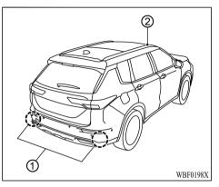
The BSW/LCA/ABSA system uses radar sensors ① installed near the rear bumper to detect other vehicles in an adjacent lane.
