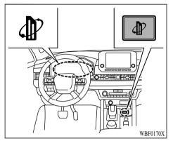
The Innovative Pedal Operation Mode will be turned ON or OFF each time the Innovative Pedal Operation Mode switch is pushed. (The Innovative Pedal Operation Mode indicator in the multi-information display shows the status of the Innovative Pedal Operation Mode.)
