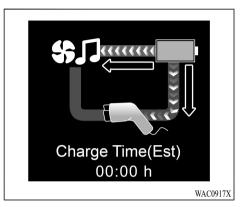
• Power is supplied from the drive battery using the V2H power supply.
