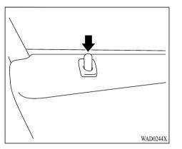
To lock the door, push down the inside lock knob.
