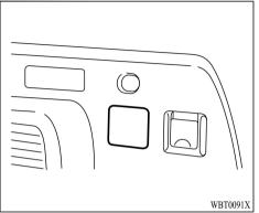
Remove the cover by inserting a flat-blade screwdriver with a cloth on the tip into the notch on the cover, on the right side of the luggage room.
