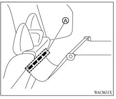
To fully cover the luggage area, affix the fasteners A on the front cover to the back of the second row seats.
