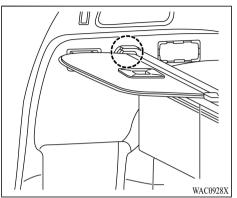
2. When not using the tonneau cover, store it with the tonneau cover inserted in the trim as shown in the illustration.
