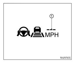
When the SET- switch is pushed down under the following conditions, the MI-PILOT Assist system cannot be set and the vehicle set speed indicator (1) blinks for approximately 2 seconds.
