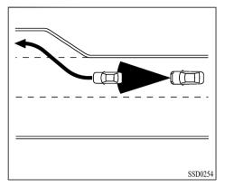
When driving on the highway at a vehicle set speed and approaching a slower traveling vehicle ahead, the ACC system adjusts the speed to maintain the distance, selected by the driver, from the vehicle ahead. If the vehicle ahead changes lanes or exits the highway, the ACC system accelerates and maintains the vehicle set speed. Pay attention to the driving operation to maintain control of the vehicle as it accelerates to the set speed.
