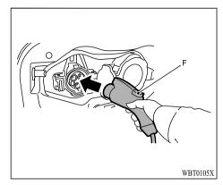
5. Without pressing the release button (F), insert the normal charge connector until a click is heard.
