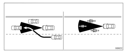
The detection zone of the ACC sensor is limited. A vehicle ahead must be in the detection zone for the vehicle-to-vehicle distance detection mode to maintain the selected distance from the vehicle ahead.
