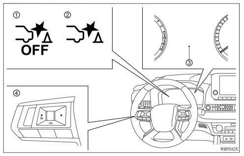
If a risk of a collision with an obstacle is detected when your vehicle is backing up, the Rear AEB system warning indicator ② will flash in the multi-information display ③ and the system will chime three times. The system will then automatically apply the brakes. After the automatic brake application, the driver must depress the brake pedal to maintain brake pressure.
