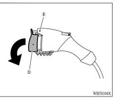
4. Open the cap (D) on the normal charge connector (E) and make sure that there is no foreign matter such as dust at the end of the normal charge connector and the normal charge port.
