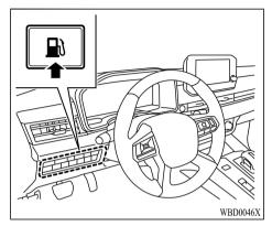
2. The fuel filler door is located on the rear left side of your vehicle.
