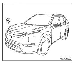
The PFCW system uses a radar sensor located on the front of the vehicle to measure the distance to a second vehicle ahead in the same lane.
