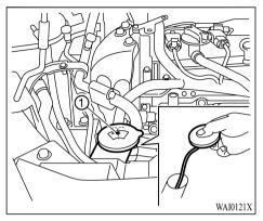
To check the fluid level, use your finger to plug the center hole ① of the cap/tube assembly, then remove it from the reservoir. If there is no fluid in the tube, add fluid.
