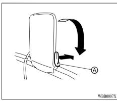
2. Push the lever (A) and fold the head restraints.
