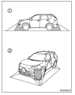
There are some areas where the system will not show objects and the system does not warn of moving objects. When in the front or the rear view display, an object below the bumper or on the ground may not be viewed ①. When in the bird's-eye view, a tall object near the seam ② of the camera viewing areas will not appear in the monitor. The following are operating limitations and do not represent a system malfunction:
