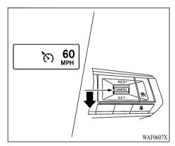
To set cruising speed, accelerate your vehicle to the desired speed, push down the SET- switch and release it. (The color of the cruise indicator changes to green and set vehicle speed indicator comes on.) Take your foot off the accelerator pedal. Your vehicle will maintain the set speed.
