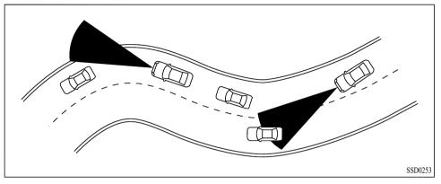
When driving on some roads, such as winding, hilly, curved, narrow roads, or roads which are under construction, the ACC sensor may detect vehicles in a different lane, or may temporarily not detect a vehicle traveling ahead. This may cause the ACC system to decelerate or accelerate the vehicle.
