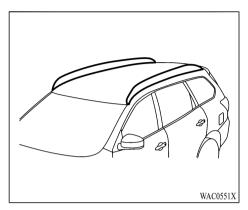
Do not apply any load directly to the roof side rails. Cross bars must be installed before applying load/cargo/luggage to the roof of the vehicle. Mitsubishi Motors genuine accessory cross bars are available through a certified Mitsubishi EV dealer. It is recommended that you visit a certified Mitsubishi EV dealer for additional information.
