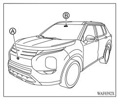
The FCM system uses a radar sensor (A) located on the front of the vehicle to measure the distance to the vehicle ahead in the same lane.
