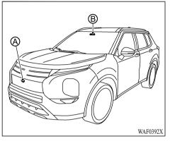
The MI-PILOT Assist system is intended to enhance the operation of the vehicle when following a vehicle traveling in the same lane and direction.
