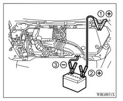
10. Connect another booster cable ③ to the negative terminal of the rescue vehicle battery.
