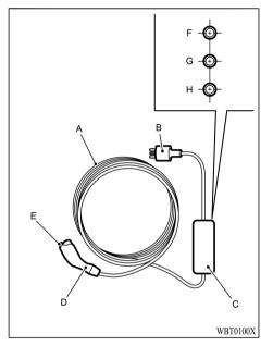
Your vehicle is equipped with a normal charging cable (AC 120V, 21 ft (6.4m)) in the bag in the cargo area.
