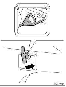
2. Unlock the charging lid by inserting a jack bar or the similar, and pulling the yellow rod in the direction of the arrow.
