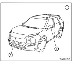
To display the multiple views, the Multi Around Monitor system uses cameras ① located in the front grille, on the vehicle's door mirrors and one just above the vehicle's license plate.
