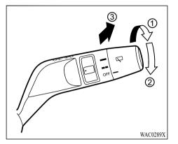
The rear window wiper and washer operate when the power switch is in the ON position.
