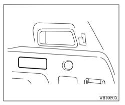
1. Remove the cover by inserting a flatblade screwdriver with a cloth on the tip into the notch on the cover, on the right side of the luggage room.
