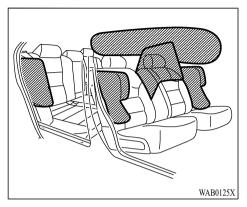
FRONT AND SECOND ROW SEAT-MOUNTED SIDE AIR-BAG, FRONT SEAT-MOUNTED CENTER AIRBAG AND SIDE CURTAIN SRS AIRBAG SYS-TEMS
