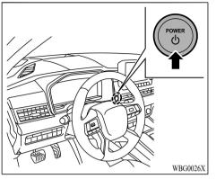
Turn off the power switch of your vehicle. (See "Power switch" (P.7-13).)
