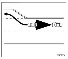
When driving on the highway at a set speed and approaching a slower traveling vehicle ahead, the ACC system will adjust the speed to maintain the distance, selected by the driver, from the vehicle ahead. If the vehicle ahead changes lanes or exits the freeway, the ACC system will accelerate and maintain the speed up to the set speed. Pay attention to the driving operation to maintain control of the vehicle as it accelerates to the set speed.
