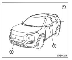
If dirt, rain or snow accumulates on any of the cameras ①, the Multi Around Monitor may not display objects clearly. Clean the camera by wiping with a cloth dampened with a diluted mild cleaning agent and then wiping with a dry cloth.
