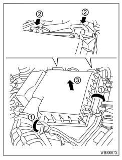
To remove the filter, release the lock pins  $\bigcirc$ , remove the stoppers from their fittings by sliding the air cleaner filter cover  $\oslash$  and pull the air cleaner filter cover upward  $\bigcirc$ .
