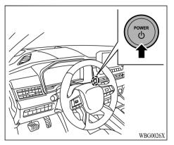
When the power switch is pushed without depressing the brake pedal, the power switch will illuminate.
