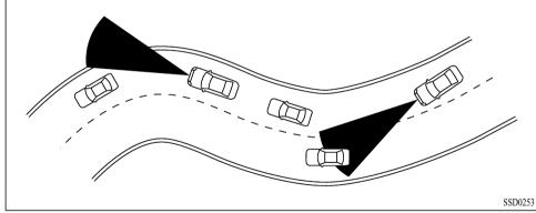
When driving on some roads, such as winding, hilly, curved, narrow roads, or roads which are under construction, the radar sensor may detect vehicles in a different lane, or may temporarily not detect a vehicle traveling ahead. This may cause the ACC system to decelerate or accelerate the vehicle.
