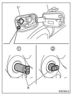
\*: The normal charge port (C) is on the left side when you are facing the vehicle.
