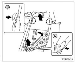
6. Remove the fuse box cover as follows.
