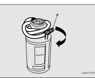
9. Pull out the compressor's hose (G) from the bottom of the compressor and securely attach it to the valve (H) of the bottle by turning it clockwise until tight.
