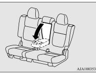
To return the seat, slide the entire seat backward to the desired position and then raise the seatback until it locks securely.
