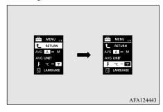
3. Press and hold the multi-information meter switch (for about 2 seconds or more) to change in sequence from  ${}^{\circ}F \rightarrow$  $^{\circ}C \rightarrow ^{\circ}F$ .
