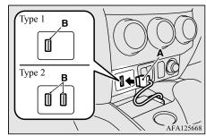
4. To remove the connector cable, turn the ignition switch to the "OFF" position or put the operation mode in OFF first and perform the installation steps in reverse.
