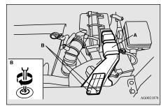
2. Turn the upper cover over. Squeeze the head of the moulding clip (C) with pliers and remove the moulding.
