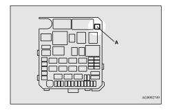
3. Clamp it on the fuse you wish to remove, and pull the fuse straight out from the fuse block.
