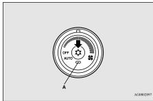
Push the switch again and the air conditioning compressor will stop and the indicator
