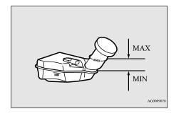
The fluid level falls slightly with wear of the brake pads, but this does not indicate any abnormality.
