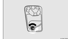
3. Turn the socket counterclockwise to remove it.
