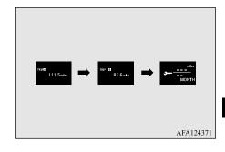
2. Press and hold the multi-information meter switch (for about 2 seconds or more) to display "-" and make it flash. (If there is no operation for about 10 seconds with this indicator flashing, the display returns to the previous screen.)
