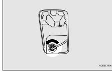
4. Pull the bulb out of the socket.
