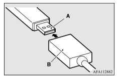
3. Connect the USB connector cable (B) to the USB input terminal (C).
