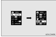
3. Press and hold the multi-information meter switch for about 2 seconds or more to switch in sequence from 1 (turn signal sound 1)  $\rightarrow$  2 (turn signal sound 2)  $\rightarrow$  1 (turn signal sound 1).
