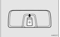
The brightness of the sunshade illumination can be adjusted to 3 different levels when the ignition switch or the operation mode is in ON or ACC.
