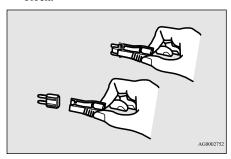
4. Use the fuse location diagrams and the matching tables, to check the fuse that is related to the problem. If the fuse is not blown, something else must be causing the problem. Have the system inspected by your authorized Mitsubishi Motors dealer or a repair facility of your choice.
