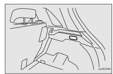
The light illuminates when the liftgate is opened, and goes out when the liftgate is closed.
