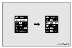
3. Press and hold the multi-information meter switch (for about 2 seconds or more) to switch in sequence from ON (operation sound on)  $\rightarrow$  OFF (operation sound off)  $\rightarrow$  ON (operation sound on). The setting is changed to the selected condition.
