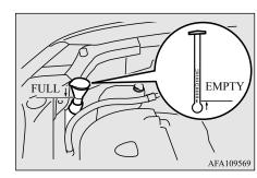
When freezing weather is anticipated, flush out the water in the reservoir by operating the pump. Fill the reservoir with windshield antifreeze (not radiator antifreeze), and operate the system for a few seconds to flush out the residual water.
