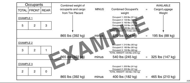
• Under a maximum loaded vehicle condition, gross axle weight ratings (GAWR's) for the front and rear axles must not be exceeded. For further information on GAWR's, vehicle loading, see the "Specifications" section of this manual.
