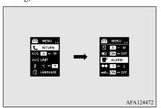
3. Press and hold the multi-information meter switch (for about 2 seconds or more) to display "ALARM" (rest time setting).
