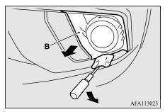
Except for vehicles equipped with daytime running lights, when unfastening the screws, be careful not to move the beam position adjustment screw (D).
