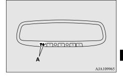
1. Within 5 seconds after successfully programming the garage door opener (refer to "Programming a new HomeLink®" section), both garage door operation indicators (A) will flash rapidly green indicating that the garage door feedback has been enabled.
