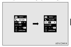
3. Press and hold the multi-information meter switch (for about 2 seconds or more) to switch in sequence from A or 1 (Auto reset)  $\rightarrow$  M, 2 or P (Manual reset)  $\rightarrow$  A or 1 (Auto reset).
