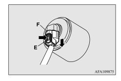
2. Insert a straight blade (or minus) screwdriver with a cloth over its tip into the light cover (B) and pry gently to remove it.
